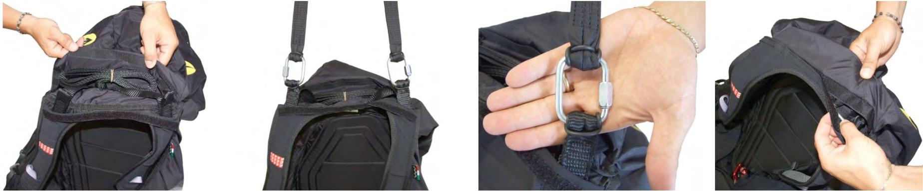
The two connections should be made using screw-lock karabiners with a breaking strength of at least 1,400 kg. In any case, it is important to verify that the length of the bridle is sufficient to position the reserve parachute inside the harness pocket, and that there is sufficient play to enable the parachute to be taken out of the pocket without causing the reserve parachute deployment bag itself to open during extraction.
