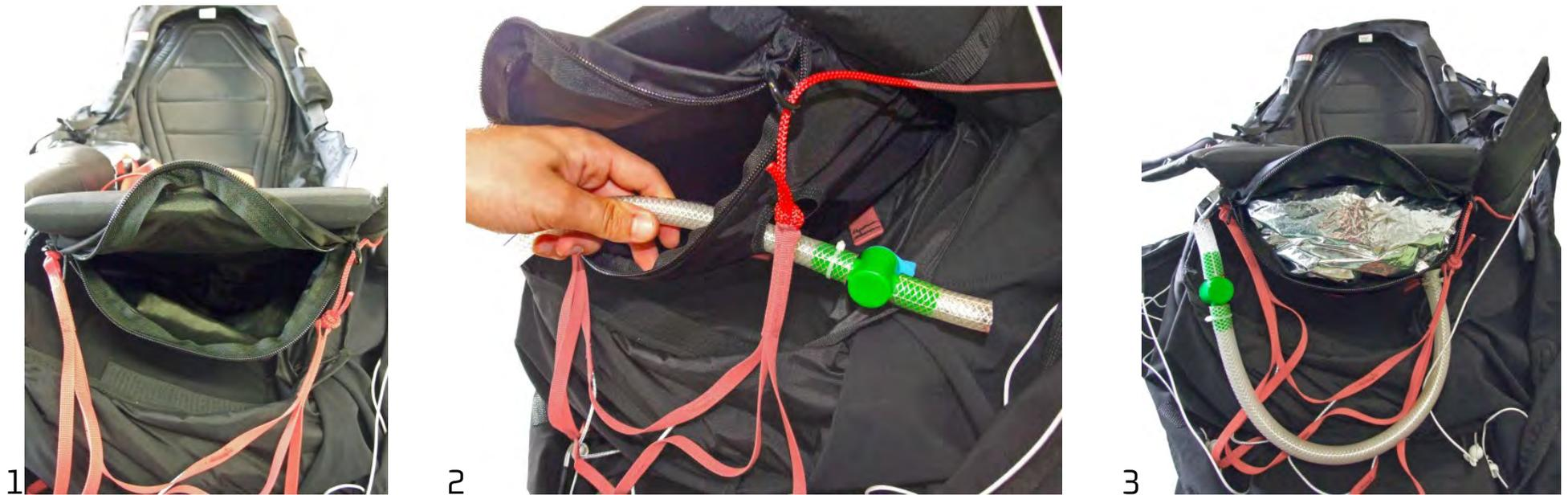
The ballast lodging is located beneath the seat. Open the zipper to access (1) the lodging, insert the discharge tube into the through-hole on the right (2) and install the ballast (3).
