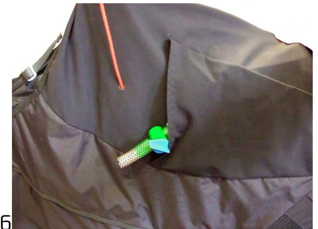
Open the zipper beneath the instrument compartment (1) to access the ballast lodging (2). Next, open the Velcro over the discharge tube's outlet hole (3) and insert the tube (4). There is a second through-hole (5) inside the harness, which allows the discharge tube to be inserted into the external pocket, where it can be hidden and extracted whenever necessary (6).
